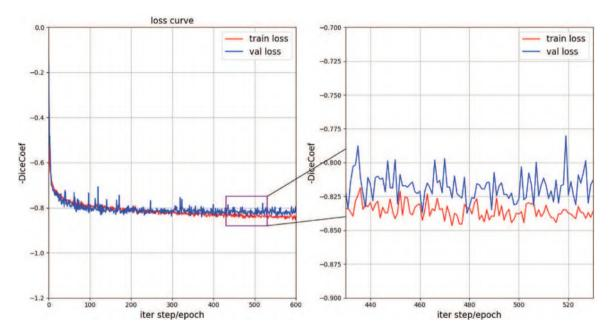
Fig. 5. The loss curve and its local enlarged curve for both training set and validation set in training process.
